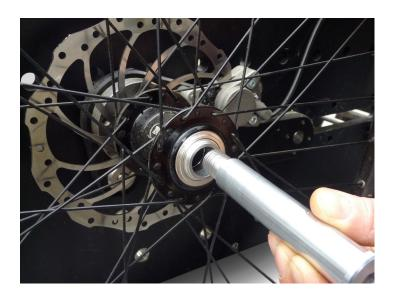
To remove the wheels, jack up the *RICKSHAW DOLLY* <sup>®</sup>. Hold the wheel in place and loosen the wheel bolt with a Size 8 Allen wrench.
